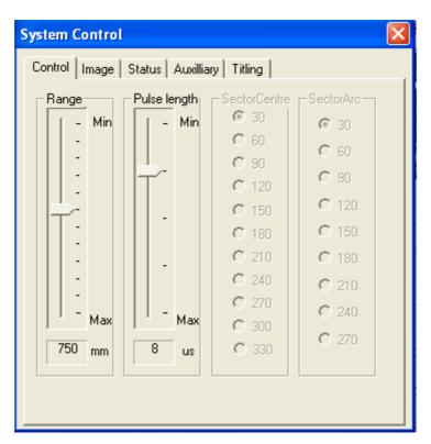
The range may be set from 125mm to 6000mm (5in to 240in) in the following settings. Note: The Sonar must be connected and running to change the range.
