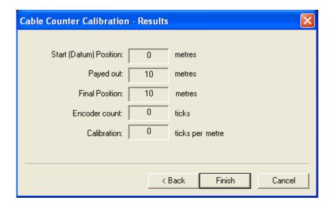
The final window in the calibration procedure shows the start and end measurements, the number of ticks counted by the cable counter, and the calibration value calculated for the cable counter.
