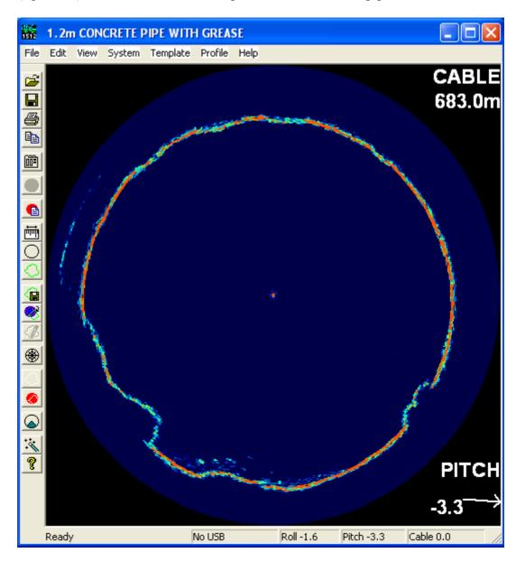
The image below shows a concrete pipe where the crown has collapsed into the invert.
