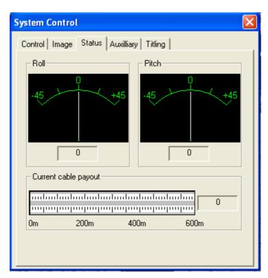
The pitch is displayed in degrees, with positive pitch indicating the sonar is pointing up.
