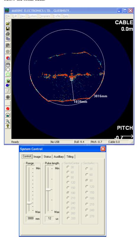
These 2 identical pictures show a fully surcharged Victorian brick sewer in which the invert has collapsed and filled with silt. The overlay circle shows where the pipe invert should be and the cursor tool the depth of collapse.
