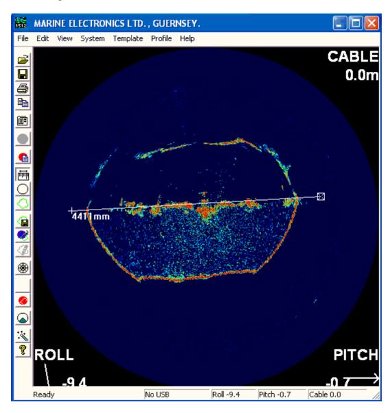
The previous image now has all the clutter removed from the screen by increasing the threshold control. This has the effect of a gain control and removes the weaker targets. The overlay circle shows the pipe diameter and the cursor tool the depth of water below the sonar head.
