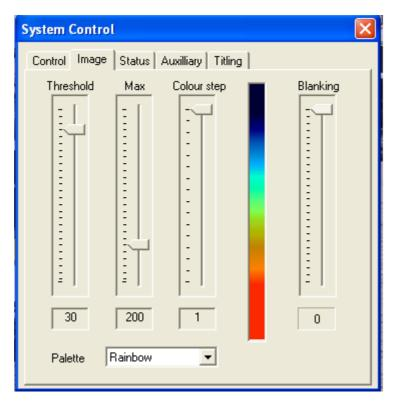
The acoustic data is collected using an 8-bit analogue to digital converter, which means raw signals are in the range 0 to 255. The colour bar to the right of the page shows the current colour scale being used, with the colour for 0 signal at the top, and that for full signal (255) at the bottom.
