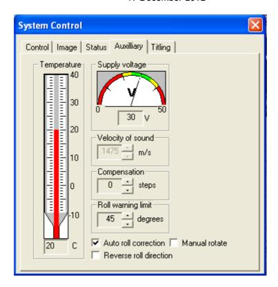
The temperature inside the sonar tool is displayed in degrees Celsius only on earlier systems with electrolytic tilt sensors. All new systems have solid-state tilt sensors which no longer support the temperature function.
