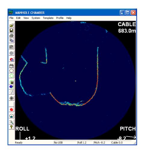
The image below of a fully surcharged brick egg shaped sewer shows a lateral entering at the top right hand side. The signal to the left, appearing outside of the pipe, is a reflection and should be ignored.
