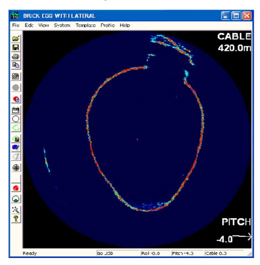
The image below shows a concrete pipe that has a build up of material on the pipe walls. It can be seen from the image that the signal strength of the reflected signal (light blue) from the material build up is much less than the pipe wall.
