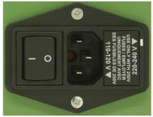
The picture shows the voltage selection set to 240v ac. To change to 110v ac remove the fuse holder and re-insert with the 110v arrow pointing towards the white line.
