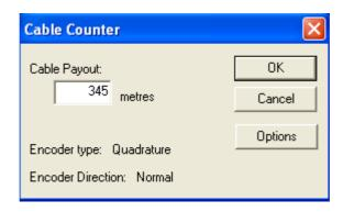
The system can operate with either a Pearpoint or Quadrature cable counter, operating in either direction. The cable counter is calibrated by running off a known length of cable. Once calibration has been performed, the system records the results and recalibration should not be necessary. ( see section 4.10 )
